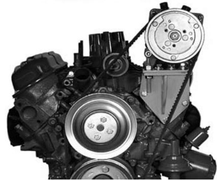
A/C bkt for Small Block Ford - Driver's Side, fits 289, 302, & 351 Windsor 105L
